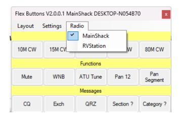
multiFlex allows multiple programs to access a Flex 6x00 radio and provide services similar to SmartSDR. Currently, a maximum of two programs (stations) is allowed. On receive they can operate independently (band, mode, etc.). On transmit, only one has control.
