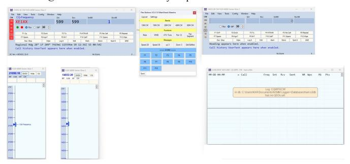
In the above picture an N1MM setup for SO2R and Flex Buttons in the middle showing a blue banner and buttons at the bottom. The banner text is "<<<< N1MM <<<<". Indicating that Flex Buttons is looking at the left (Slice 1) screen for action. Clicking on the banner will change the text to ">>>> N1MM >>>>" indicating Slice 2.
